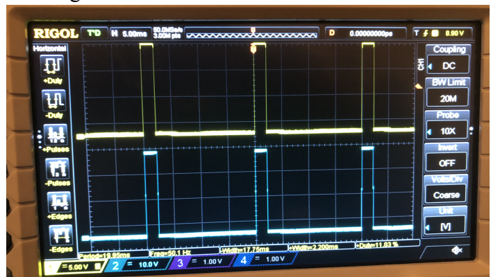
Figure 13. PWM Signal Display [22]
